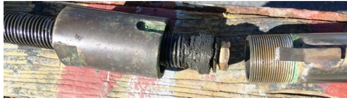
our 5 years old system. There was water in the lower tube
